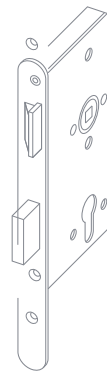
DIN right hand lock (the straight side of the latch points to the right)
